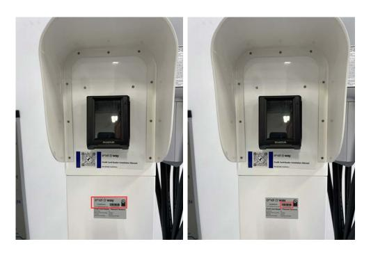
2. Locate the serial number label on the bottom side of the new CCR and record the CCR and ICCID numbers from the label.
