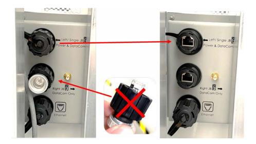
3. Connect the left JuiceBox serial cable to the top RJ45 adapter and right JuiceBox serial cable to the middle RJ45 adapter on the back cover of the CCR assembly. Turn the cable connectors clockwise until they are latched.
