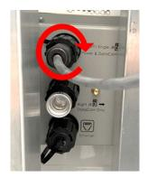
3. Connect the SMA plug from the antenna to the SMA bulkhead on the back of the CCR cover and make sure the connection is tight.
